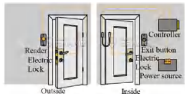
Fig. 1. Principle of electric locks operation
