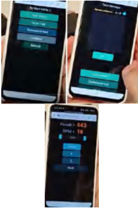
Fig. 2. The interface of the developed application for the quality assessment system of the brushless DC motors
