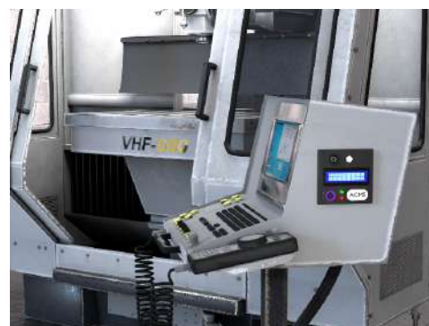
Figure 2. - Access Control System on the Equipment
