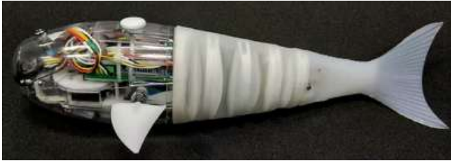
Figure 6. – Zoomorphic mobile robot fish Jiayong Chen[15]
